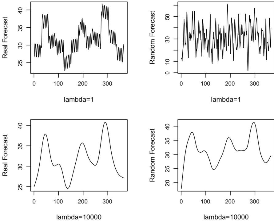
**Fig. 2** Showing four different PFCs constructed by the method described in Fleten and Lemming (2003), two curves made with a forecast from dummy variables and two curves where the forecast is just drawn from a normal random variable, with  $\lambda = 1$  and  $\lambda = 10,000$
